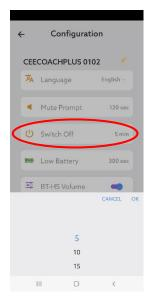
(i) In the delivery state or after a reset of your device, the value for the automatic switch-off is 5 minutes.
