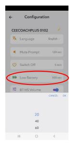
(i) In the delivery state or after resetting your device to the default state, the value is 300 seconds.
