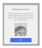
► Confirm the connection request on your device with a short press (less than 1 second) on the function key (1).
